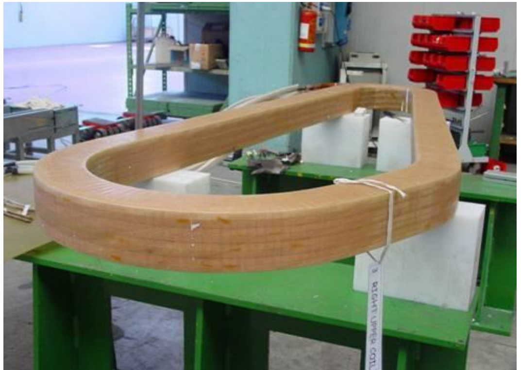
Lateral coil after impregnation
